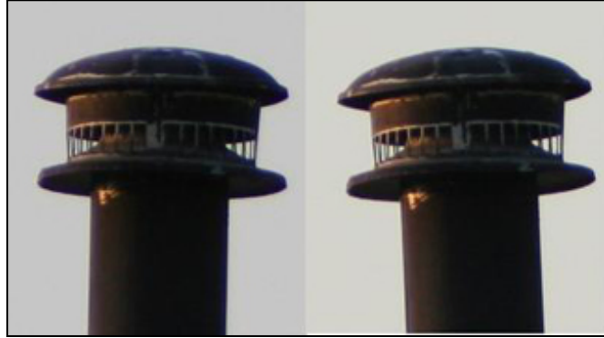
Pictures taken of the neighbor's chimney using no eyepiece and a Canon 20D. They are cropped and zoomed to 100%. Left image is without the VR-1 (violet reduction) filter, and the right is with the filter
