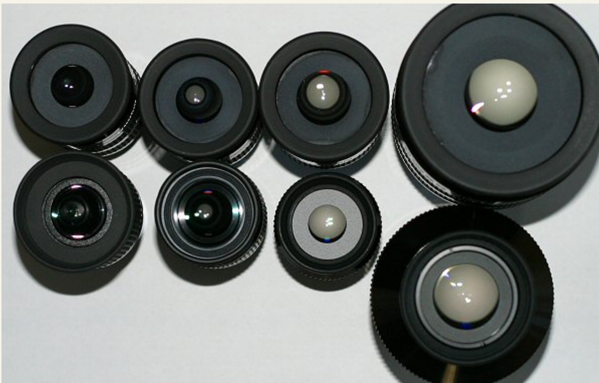
Top Row Left to Right: UWAN 4, UWAN 7, UWAN 16, UWAN 28 Bottom Row Left to Right: Burgess / TMB 4mm, Nagler 7mm t6, Nagler 16mm t5, Nagler 26mm t5 (w/ Dioptrx)
