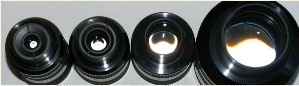
Field lens - Left to Right - 4mm UWAN, 7mm UWAN, 16mm UWAN, 28mm UWAN
