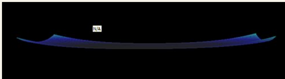
CCDInspector Visualization of the triplet's field flatness - Angle 2
