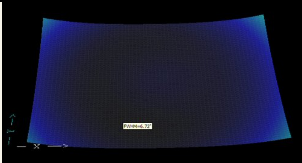
CCDInspector Visualization of the triplet's field flatness - Angle 1
