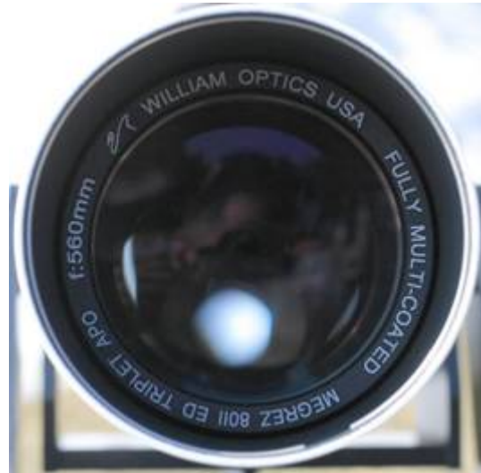
Note the lack of blackening on the dew shield retaining ring
